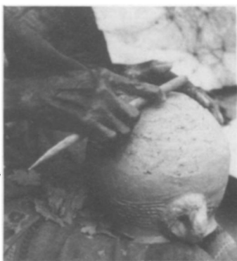
5. Scraping the bottom.
